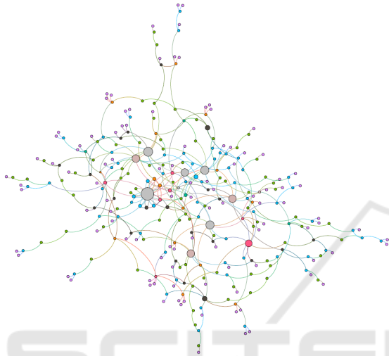
Figure 1: Visualisation of network size: 300 agents. The various colours represent the degree of each node; purple=1 connection, light green=2, blue=3, black=4, orange=5, green=6, red=7, light pink=8, grey=9 or more.
