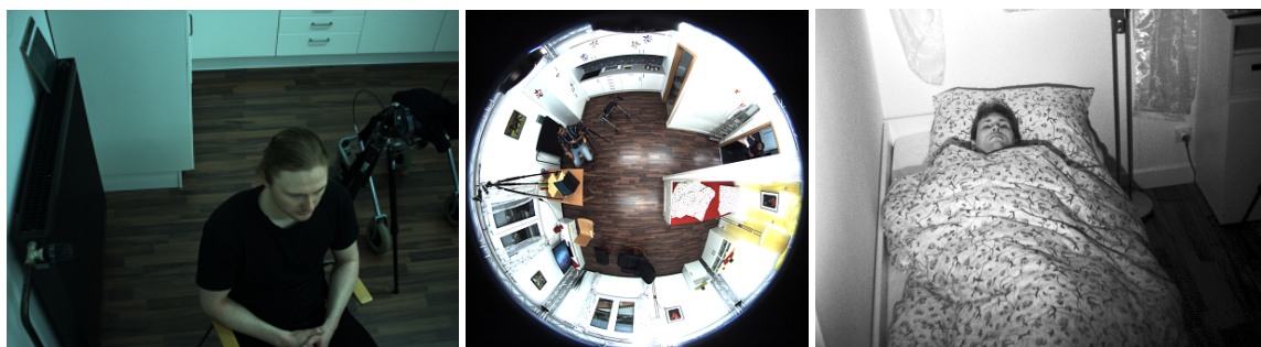
Figure 1: Different scenarios to determine the heart rate in home environments from left to right: Proband sits on a chair recorded by narrow lens camera, proband sits on a chair recorded by omnidirectional camera, proband lies in a bed recorded by monochromous camera.
