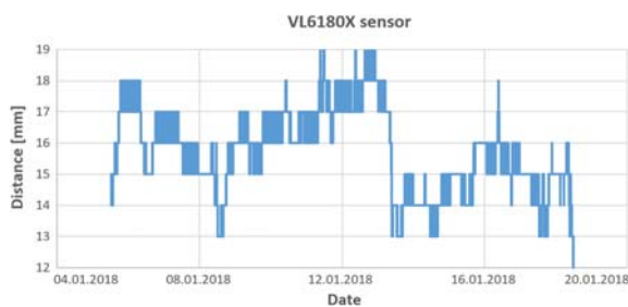
Figure 4: Continuous operating test of one of three VL6180X sensors.
