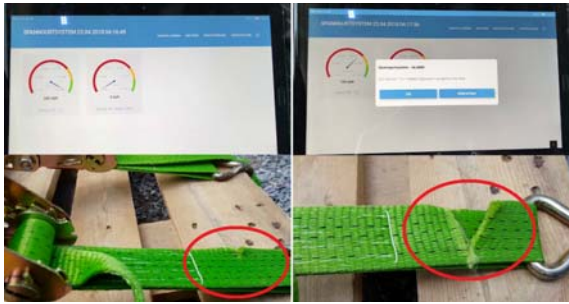
Figure 10: Alarm message during the crucial test. Left: Intact lashing belt. Right: Torn lashing belt.
