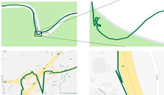
Figure 7: Filtered GPS errors with thresholds derived from the curviness and relation of GPS distance to driven distance.
