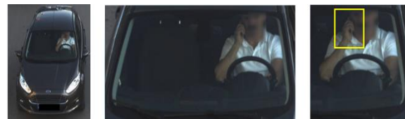
Figure 1: Steps of the proposed method. Left, middle and right column show License Plate Recognition Camera vehicle image, detected windshield region and detected driver region, respectively. Yellow rectangle shows the presence of cell phone usage within the driver region.
