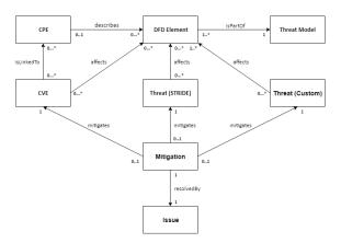
Figure 1: OVVL Conceptual Data Model.
