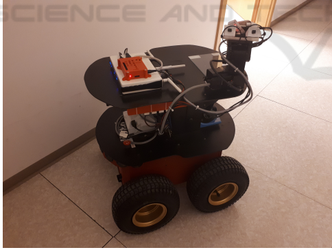
Figure 1: WMR Pioneer 3-AT with a stereo camera on a PTU.
