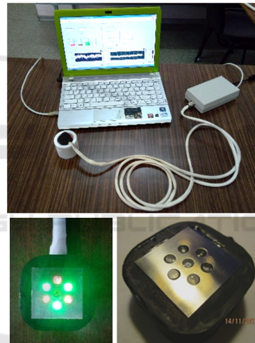
Figure 3: The appearance of the developed prototype for measuring the skin blood flow (BF).
