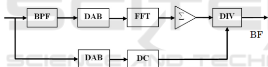
Figure 4: The block-diagram of data processing. BPF is the band-pass filter, DAB is the data accumulation buffer, FFT is the Fast Fourier Transform module, \Sigma is the adder, DIV is the divider, DC is the unit for extraction of the \langle i(t) \rangle .
