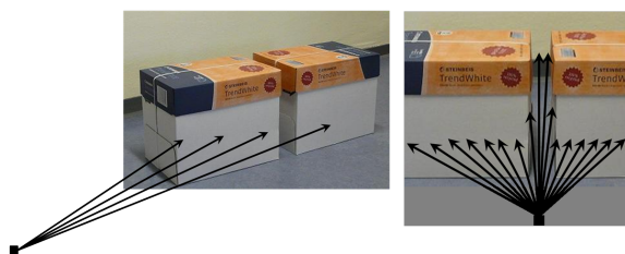
Figure 4: Relationships between incident angle of the sensor beam and point density at the surface. More dense surface sampling offers more reliable surface information.
