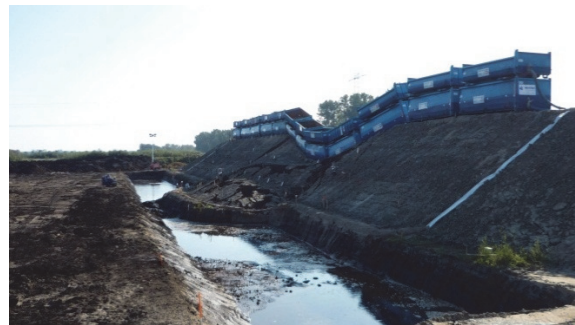
Figure 3: Dike breach of macro stability experiment (photo: TNO 2008).
