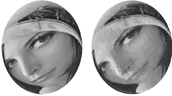
Figure 3: Compression with Bonneau spherical wavelets. Left: original; Right: reconstruction with 5% of the coefficients.
