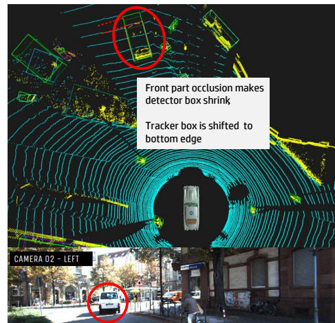
Figure 9: Instance of perspective correction. Bounding box of a self-occluded van located in front of ego-vehicle is shifted downward so that the van dimension is retained.
