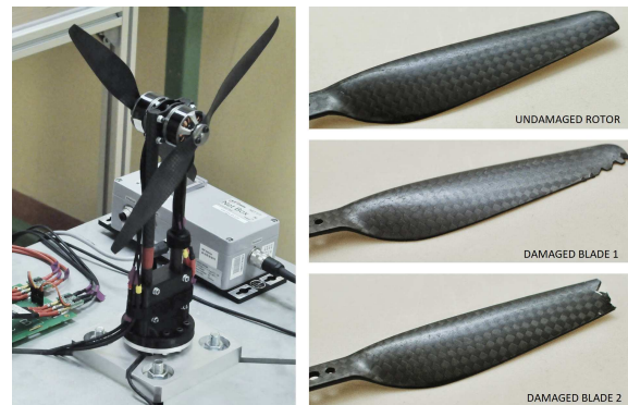
Figure 1: The propulsion test stand and set of tested rotors with different degrees of structural damage.
